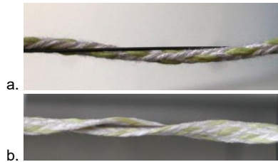
Fig. 34: Braided round (a) and flat (b) cord wound around a Ø 1.2 mm wire.
