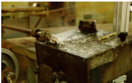
Fig. 3: Fumes released during solvent-based wire lubrication
