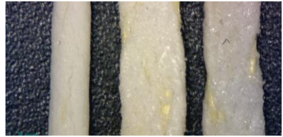
Fig. 36: Viscose-aramide-based abrasive cords with \text{Al}_2\text{O}_3 particles: round with small grains (left), flat with medium-sized grains (middle) and large grains (right)
