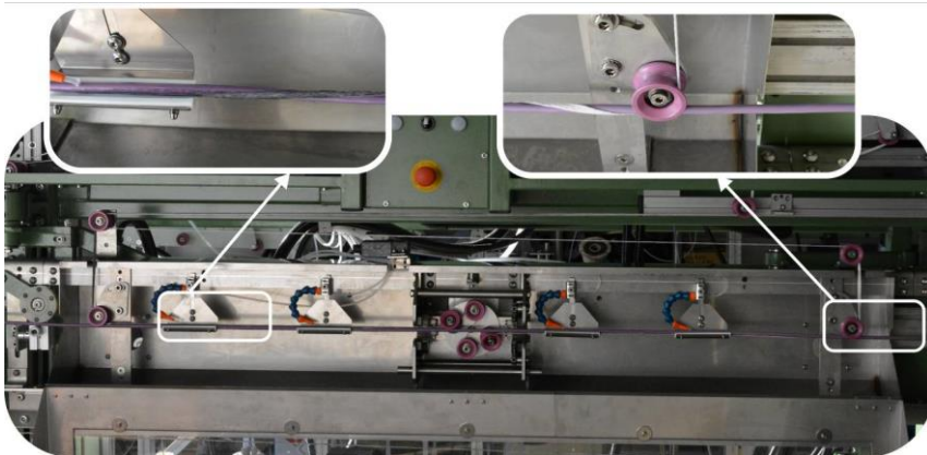
Fig. 42: HELICORD® machine NB57 with special looping unit and multiple liquid metering outlets for removal of misprints from cable jackets. Display details before (left) and after (right) removal of the misprint
