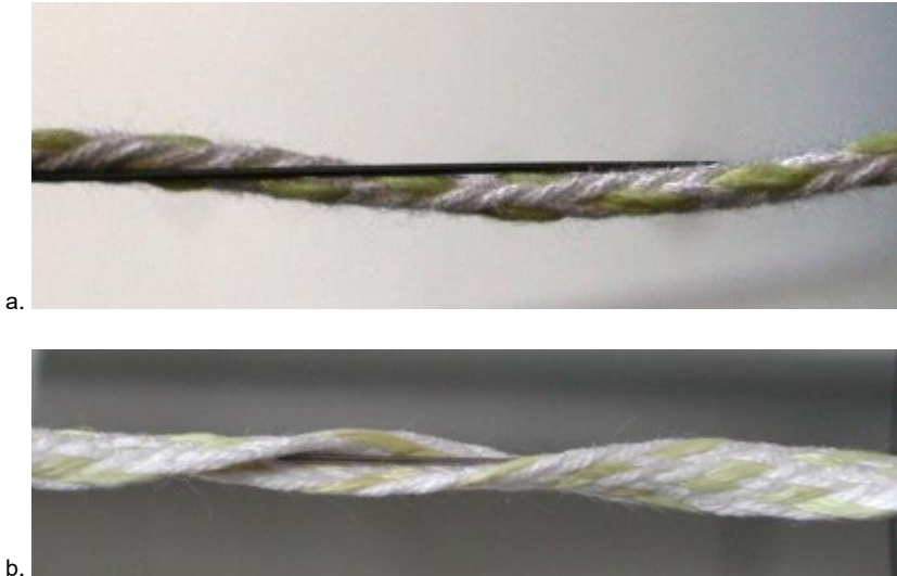
Fig. 34: Braided round (a) and flat (b) cord wound around a Ø 1.2 mm wire.
