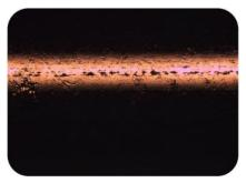
Picture 6: Surface of copper-coated welding wire ( $\emptyset$  1.18 mm) after the skim pass using NB10H038 and corrosion test
