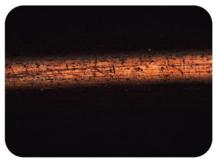
Picture 7: Surface of copper-coated welding wire ( $\emptyset$  1.18 mm) after the skim pass using a conventional dispersion and corrosion test
