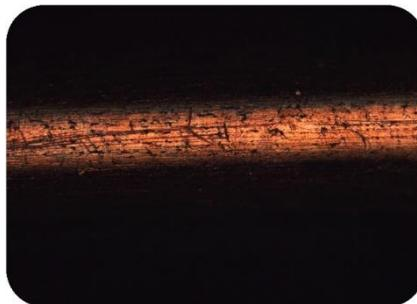
Picture 7: Surface of copper-coated welding wire (Ø 1.18 mm) after the skim pass using a conventional dispersion and corrosion test
