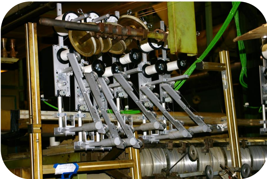
c 2009: SICME NEM; VD 60; these lubricators were supplied and supervised by a PLC-based control box NB50E606 with two-line text display, yarn slip supervision and detailed error alarm function
