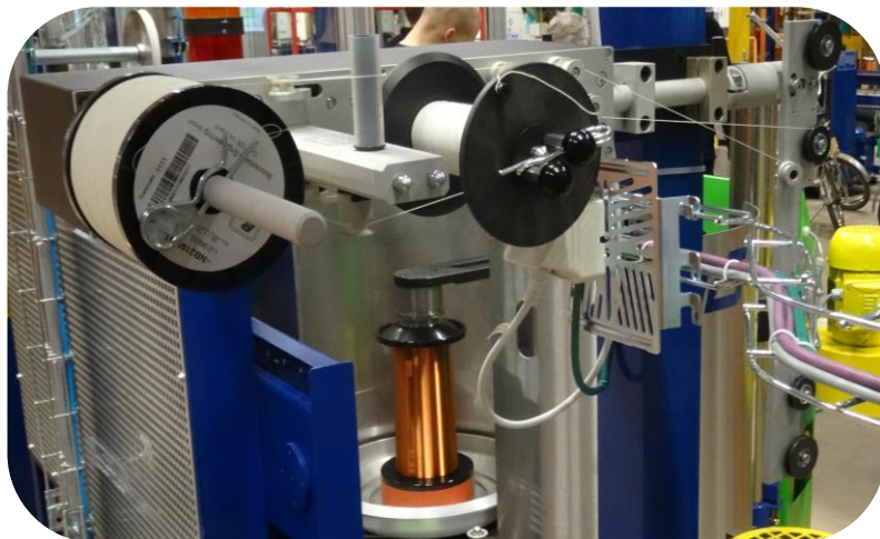
Fig. 13: NB52 (model 2016) for warm wire lubrication
