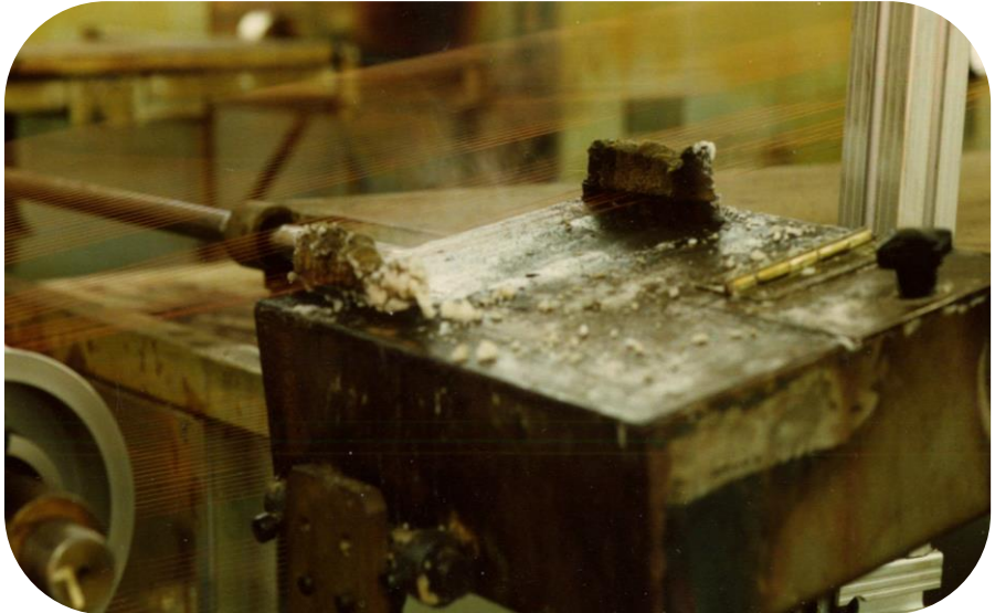
Fig. 3: Fumes released during solvent-based wire lubrication
