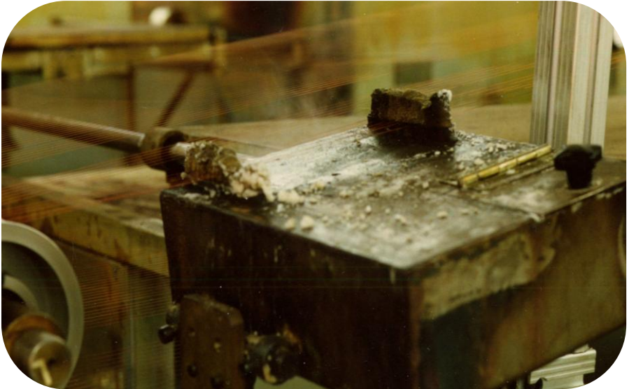
Fig. 3: Fumes released during solvent-based wire lubrication
