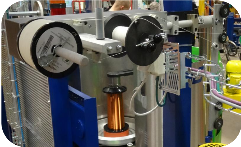
Fig. 13: NB52 (model 2016) for warm wire lubrication
